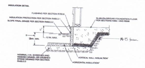
4" washed gravel or crushed stone (minimum) at highest point of bedrock Footing Depth 16"
